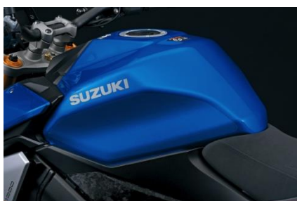
30 Fuel tank protection foil (Transparent) Protects against tank scratches
