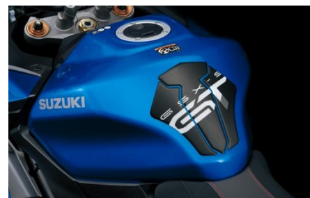
29 Fuel tank pad For tank scratch protection, features new GSX-S GT logo
