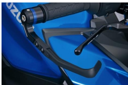
12 Brake lever guard Made of high-end billet aluminum and resistant plastic
