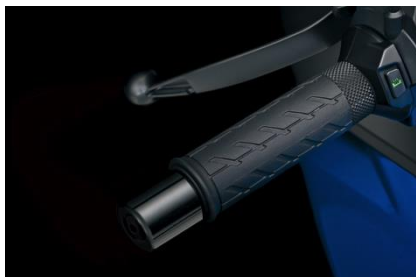
8 Grip heater With three different heat settings Entire surface is heated
